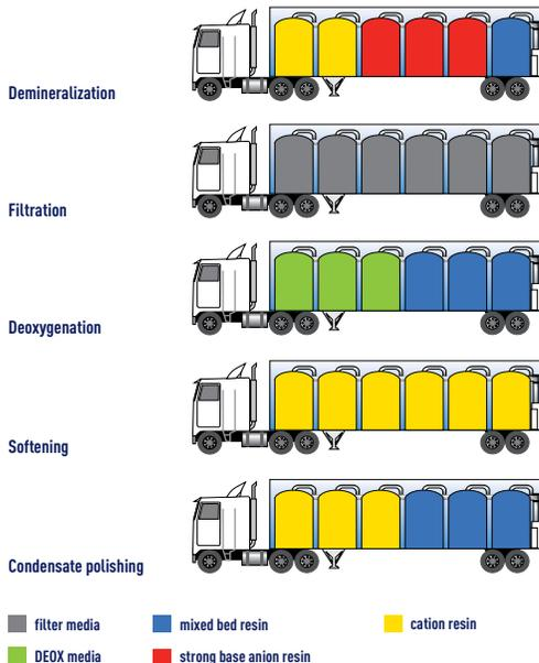
At SUEZ, we design water systems using the latest technologies suited to your specific water needs and applications. Ion exchange technology, like that used in our MobileFlow\* system, is well suited for applications such as water softening, demineralizing, and condensate polishing (reducing iron and silica content in water). See the diagram below for more information.
